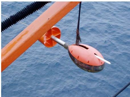
During D285 a total of 210 surface samples were collected during the cruise. Water was pumped up from the clean fish (Fig. 7.1) at a depth of ~6m and into the clean container where it was withdrawn at the manifold either un-filtered or through a 0.2  $\mu$ m filter cartridge.
