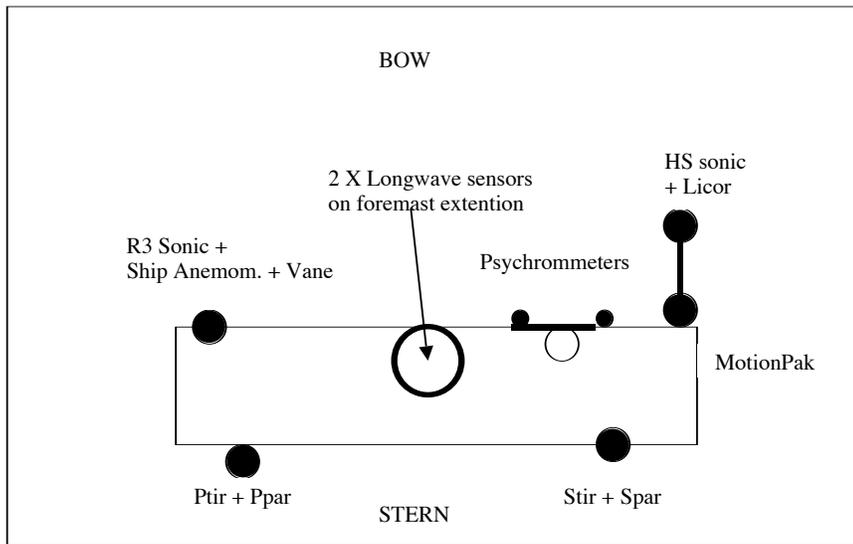
Fig. 2.2 Schematic plan view of the foremast platform, showing the positions of the sensors.
